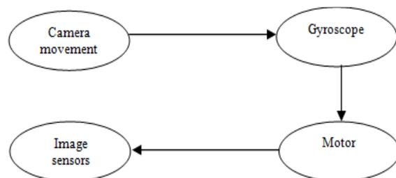
Fig. 8: Steps in optical image stabilization
