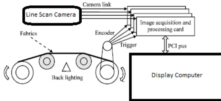
Fig. 5: Architecture of a defect detection system (image courtesy <http://sialert.net/>)
