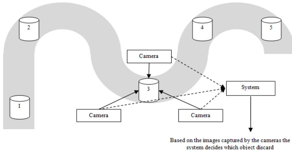
Fig. 4: Cameras at different angles to capture images of a single object moving along a production line
