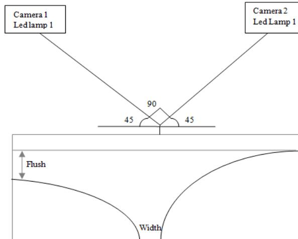
Fig. 2: Arrangement of cameras and LED lamps with respect to the object
