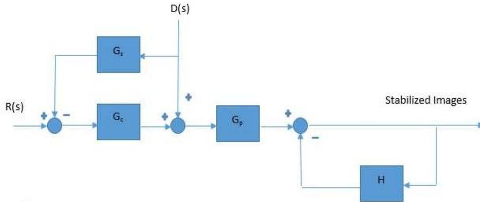
Fig. 10: Block diagram of closed loop control scheme
