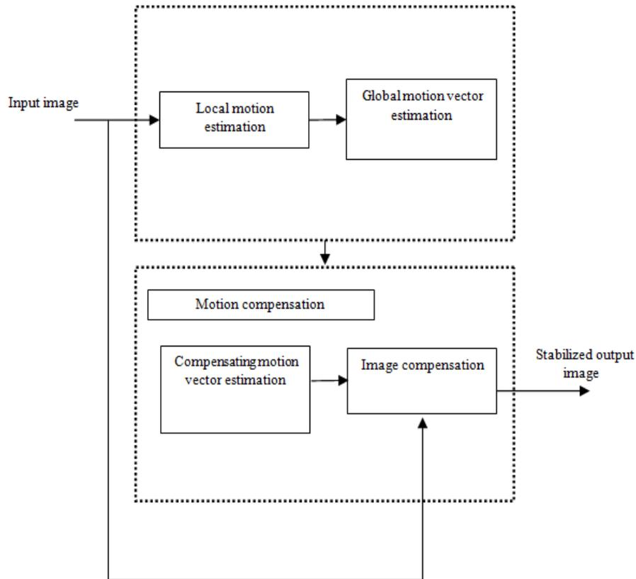
Fig. 9: DIS architecture (image courtesy: <http://cdn.intechopen.com/pdfs-wm/10608.pdf>)
