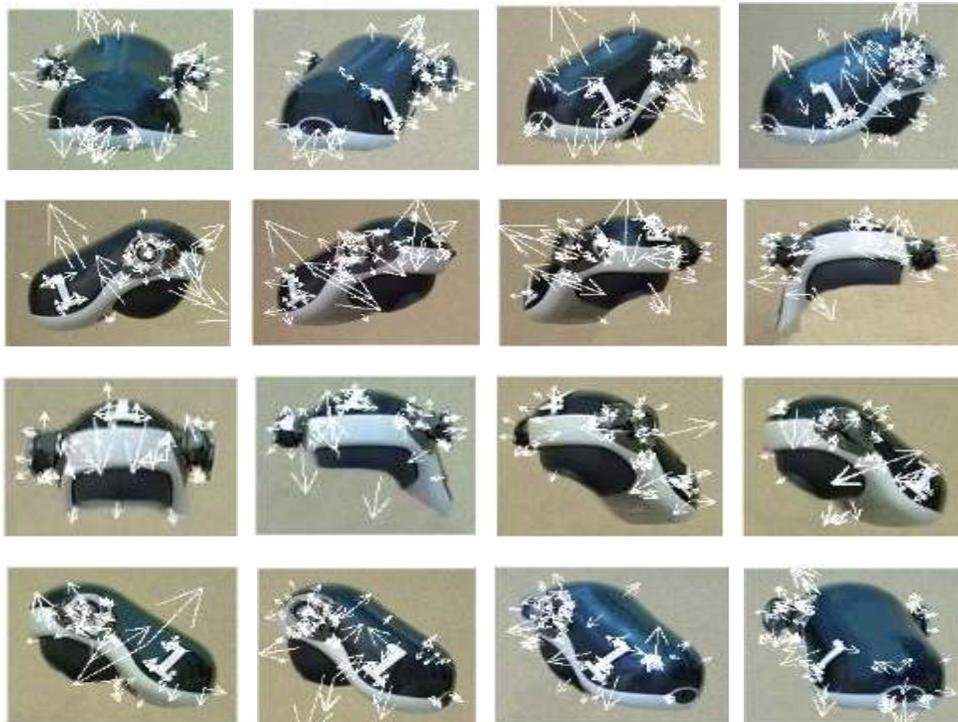
Fig. 11: Robot head prototypes with their SIFT's (image courtesy: Loncomilla and Ruiz-del-Solar (2005))
