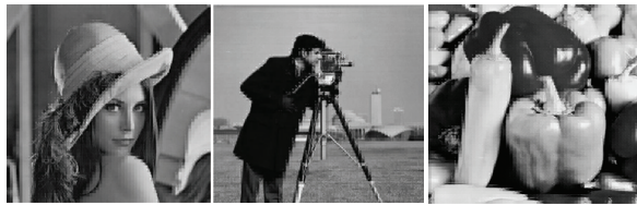
Fig. 4. Reconstructed images after thresholding Discrete Rajan Transform output ( T = 0 ; block size 8 \times 8 ).
