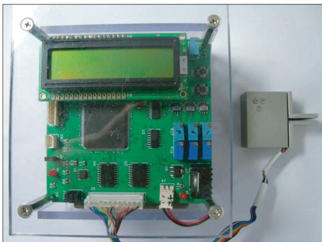
Fig. 1. Digitalized Pinch Dynamometer.
