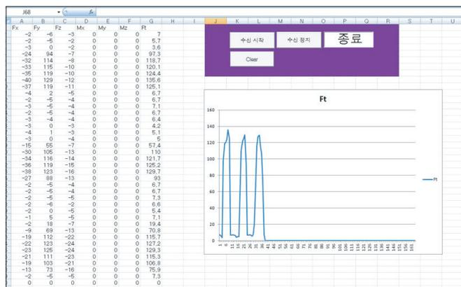
**Fig. 2.** Display window for the Digitalized Pinch Dynamometer.
