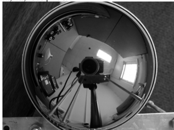
Figure 3. Photo taken by the panoramic imaging sensor with visible light.
