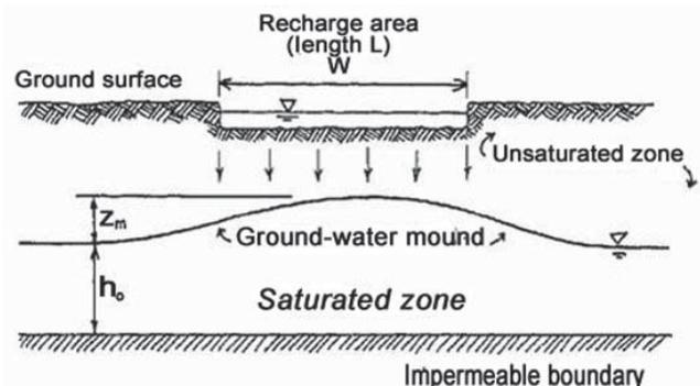
Figure 3: Diagrammatic representation of the groundwater mounding (FINNEMORE, 1995).
