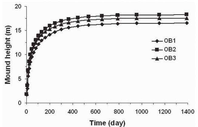
Figure 6: Height of the groundwater mound beneath the recharge basin calculated with the numerical model.
