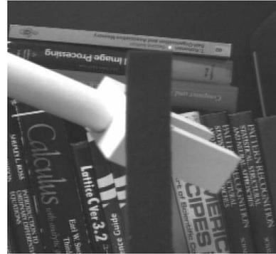
Figure 5: Shown here is an original image frame used for the motion tracking. An obstacle significantly occludes a part of the object. The complicated background also causes a difficulty in object recognition using conventional methods. This image was taken at time index 10 in Fig. 10.
