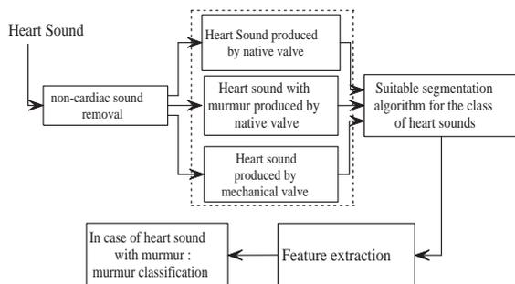
Figure 1: Main blocks for heart sound analysis framework where blocks under dotted square is for discrimination for the three groups of sounds.
