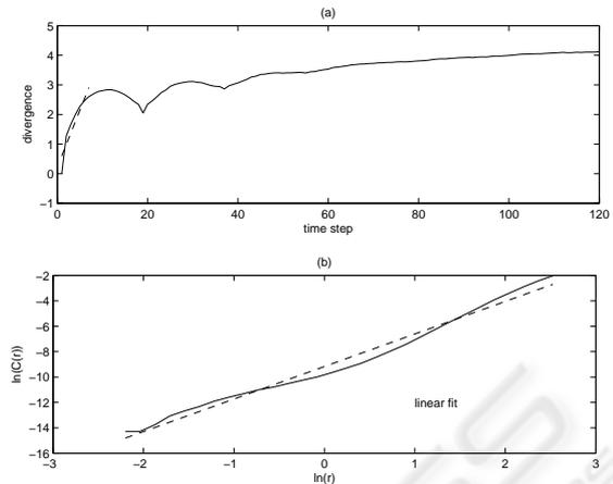
Figure 6: Embedding features computation by linear least square fitting : (a) Largest Lyapunov exponent (b) Correlation dimension.
