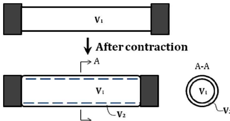
In the analysis above, the volume inside the pneumatic muscle is treated as a whole. However, one can gain further insight of the force-generating process by hypothetically dividing the internal volume into two portions, including  $V_1$ , a cylindrical volume at the center of the muscle, whose diameter is equal to that of the muscle's end connectors; and  $V_2$ , a ring-shaped volume surrounding  $V_1$  (Figure 3).
