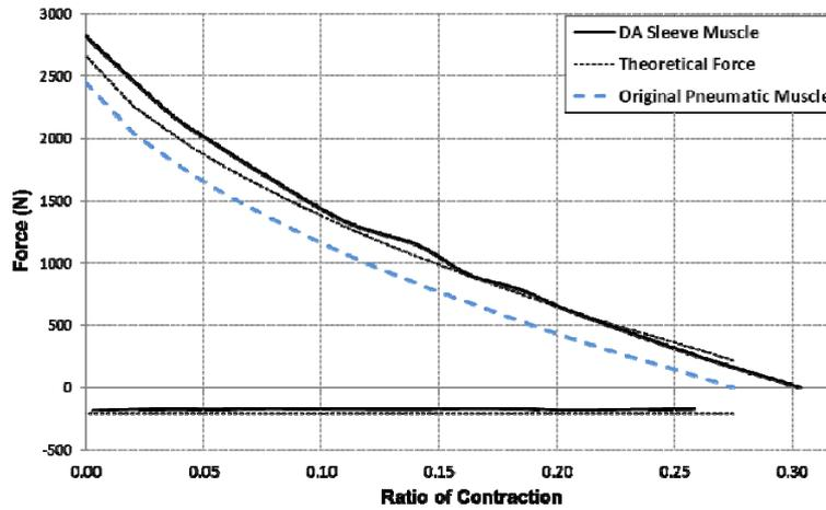
**Figure 10.** Measured and theoretically calculated force outputs of the DA sleeve muscle in comparison with the force output of the original unmodified pneumatic muscle under the gauge pressure of 414 kPa (60 PSI).
