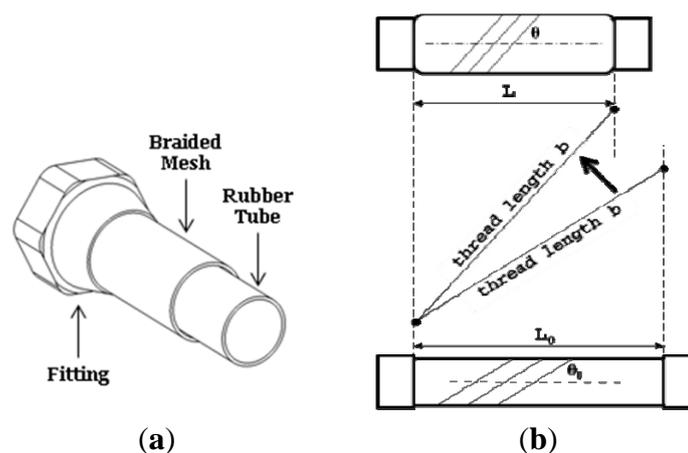
Despite the extensive robotic application, the innovation on the pneumatic muscle itself has been limited, with the flexible membrane as the major focus of investigation. For example, the bi-layer membrane structure as shown in Figure 1a can be modified into an embedded design, in which the load-bearing fibers are embedded into the flexible air-tight membrane to form a single-layer structure [14], which has been adopted in a large number of pneumatic muscle designs, including the commercial
