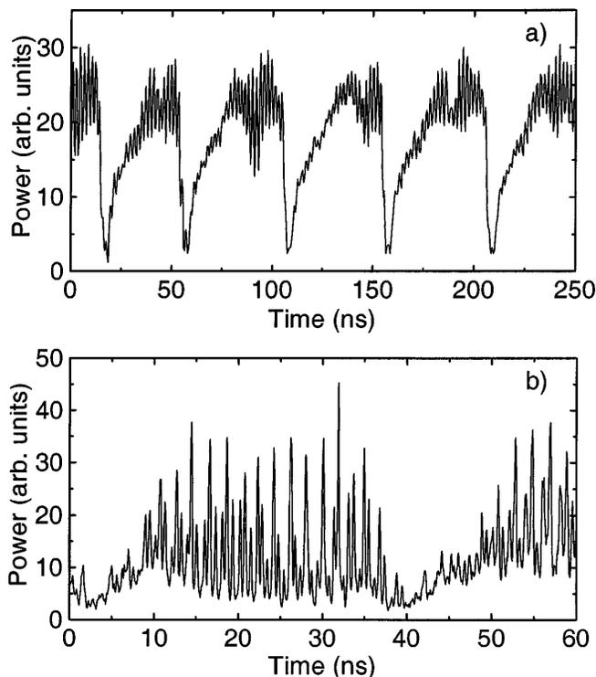
FIG. 1. Total intensity as a function of time taken with (a) the oscilloscope, and (b) the streak camera with a time resolution of about 230 ps. Note the pseudoperiodicity of the signal at the round-trip time in the external cavity ( $\sim 2$  ns).
