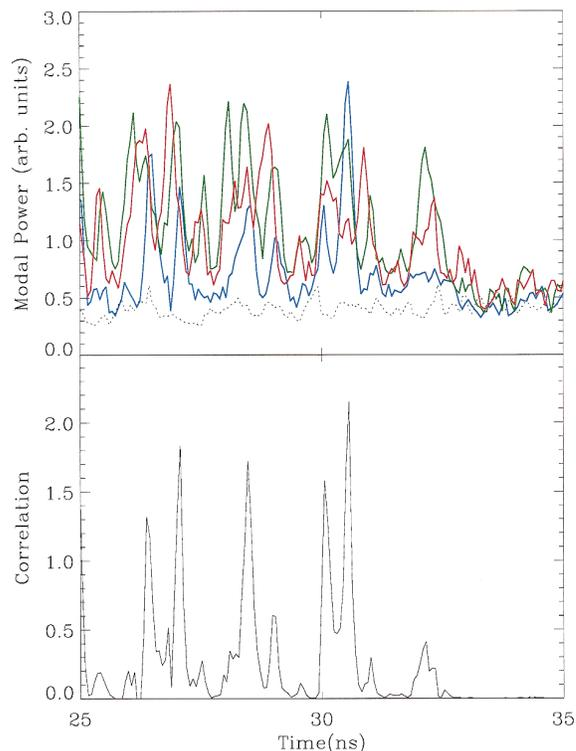
FIG. 4. Top panel (color): Modal intensity traces for the three dominant modes in Fig. 3 for times around the first drop. Blue corresponds to the mode at about  $\delta\lambda = 60$ , green to that at about  $\delta\lambda = 100$ , and red to the one at about  $\delta\lambda = 150$ . The dotted black line corresponds to the background level. Bottom panel: modal correlation defined as the product of the modal powers above the background level.
