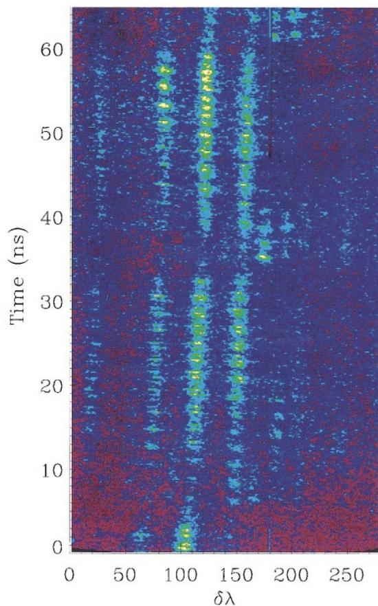
FIG. 3(color). Typical time-resolved spectrum in the LFF regime taken with the streak camera. The time span is 65 ns with a time resolution of  $\approx 230$  ps, while the frequency resolution is  $\approx 40$  GHz. The index in  $\delta\lambda$  denotes the pixel on the CCD array, and the power is in false color, from purple (low power) to bright red (high power).
