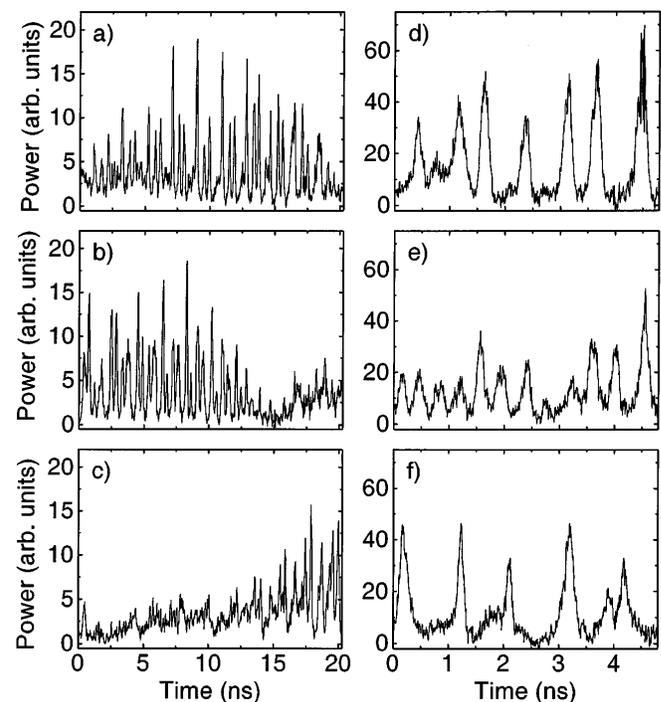
FIG. 2. Temporal evolution of the total intensity taken with the streak camera over different time spans: (a)–(c) 21 ns time span, 70 ps time resolution; (d)–(f) 4.5 ns time span, 16 ps time resolution. Different traces correspond to different drops, and the starting point relative to the drop is changing from one acquisition to the other.
