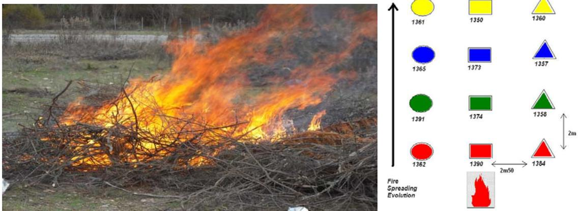
**Figure 5.** MICA 3<sup>rd</sup> GEN Experimental Area with eight sensors on a square with 2 m in width and 2 m in distance between the nodes.
