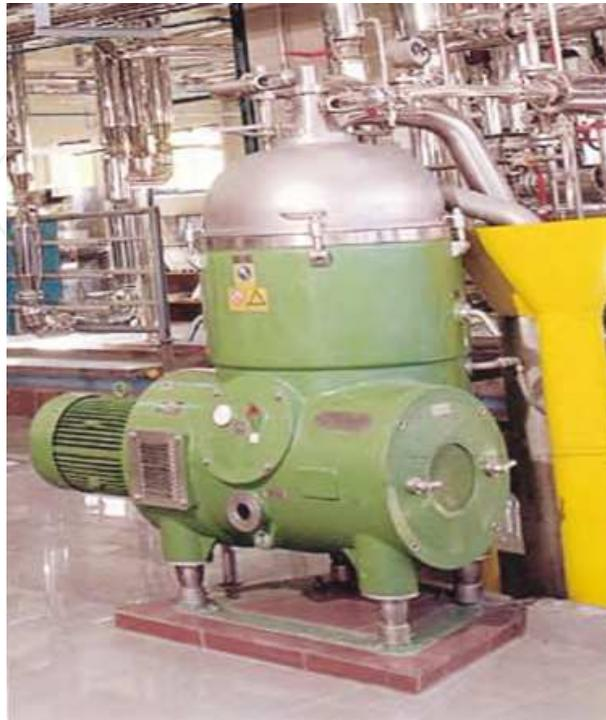
Fig. 6. Degumming Separator
