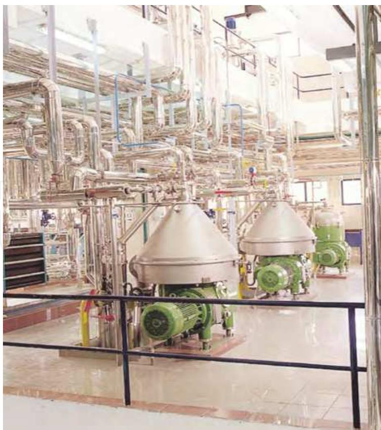
Fig. 7. Neutralization Separator
