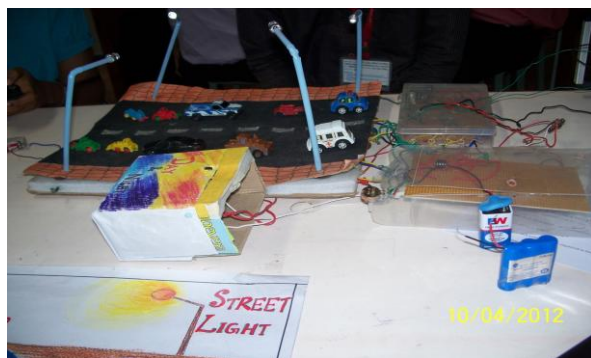
Fig.3.1.3: Implementation of the proposed work on miniature project model giving results upto 25V from a single Piezo chip. This estimates the calculation that a single human step can flicker 60W bulb for 1sec. Therefore, for a crowd in motion, multiply with 28527* times, which can move a train for 1second by calculation for a complete strip layout of Piezo material.
