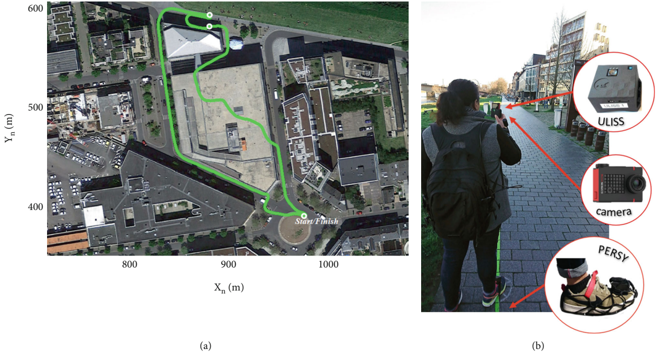
FIGURE 6: (a) IRSTV dataset path and (b) experimental setup.
