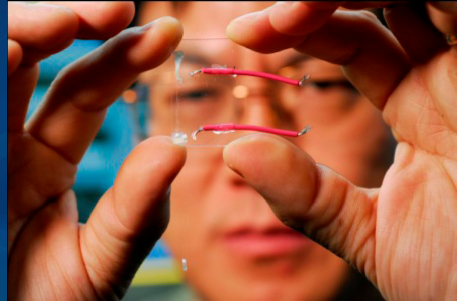
Georgia Tech Regents' Professor Zhong Lin Wang holds a prototype microfiber nanogenerator. Image Credit: Georgia Tech / Gary Meek ( ref. 2 )
