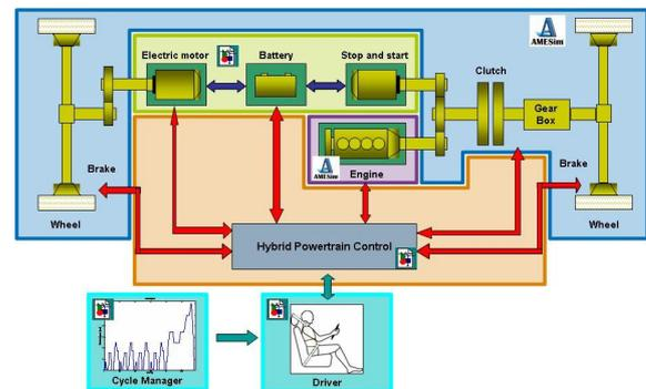
Fig. 4. Co-simulation architecture describing the involved models
