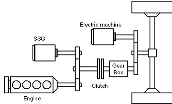
Fig. 3. The parallel hybrid architecture
