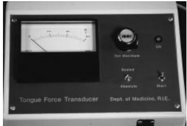
Fig. 3. – Control box with analogue scale capable of registering force in absolute units (N) or as a percentage of maximum force.
