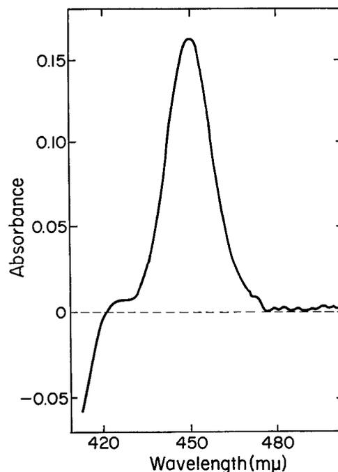
Fig. 7. Carbon monoxide difference spectrum of P-450 preparation, determined as described in the text. The protein concentration was 2.9 mg per ml.
