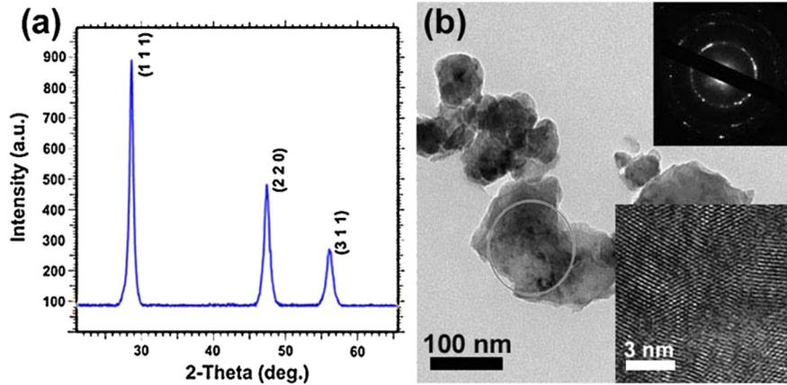
FIG. 1 (color online). XRD pattern (a), TEM image of ball milled  $\text{Si}_{95}\text{Ge}_5$  nanopowders (b). The insets to Fig. 1 (b) are the diffraction pattern and HRTEM image for the circled region.
