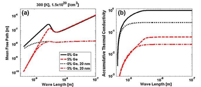
FIG. 4 (color online). Modeling results for the thermal conductivity at room temperature: (a) mean free path vs phonon wavelength and (b) accumulative thermal conductivity ratio vs phonon wavelength for different Ge ratios and grain sizes.
