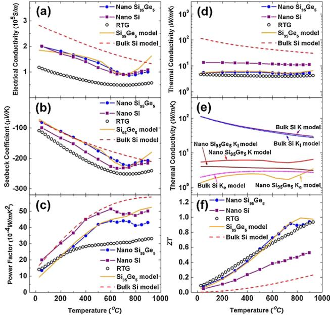
FIG. 3 (color online). Temperature-dependent electrical conductivity (a), Seebeck coefficient (b), power factor (c), thermal conductivity (d), electron ( $K_e$ ), phonon ( $K_l$ ), and total (K) thermal conductivity by modeling (e), and  $ZT$  (f) of nanostructured Si (filled squares), nanostructured  $\text{Si}_{95}\text{Ge}_5$  (filled circles for experiment and solid line for model), bulk Si model (dashed line), and  $\text{Si}_{80}\text{Ge}_{20}$  RTG samples (open circles).
