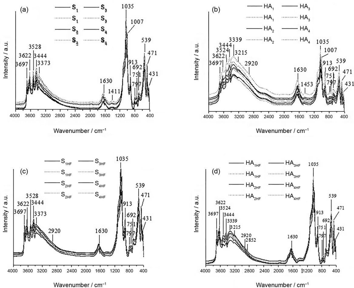
**Figure 3.** FTIR spectra obtained before the HF treatment for soil samples in (a) and HA samples in (b), and after the HF treatment for soil samples in (c) and HA samples in (d), where continuous and discontinuous lines indicate that the measurements were performed in duplicate.
