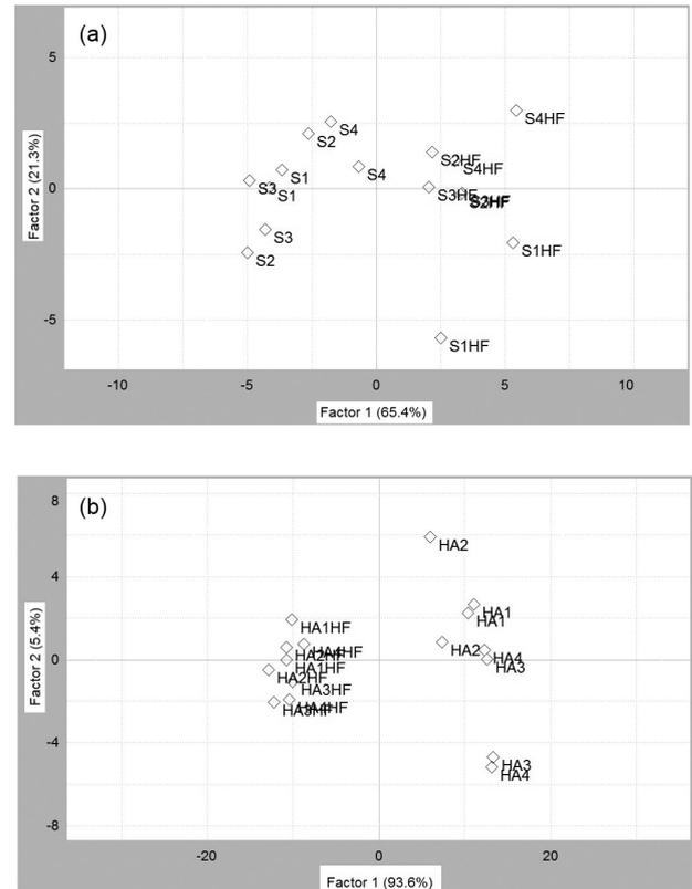
**Figure 5.** Statistical analysis graph: PC1 versus PC2 scores obtained with FTIR results of soil samples in (a) and HA samples in (b), before and after the HF treatment, at the region between 3755  $\text{cm}^{-1}$  and 2900  $\text{cm}^{-1}$ .
