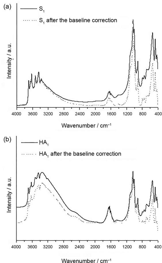
**Figure 2.** Comparison of  $S_1$  in (a) and  $HA_1$  in (b) FTIR spectra, before and after the baseline correction.
