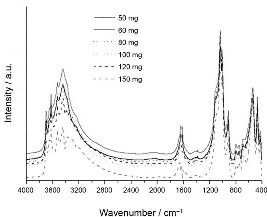
**Figure 1.** FTIR spectra obtained from the sample pellet made with 1.5 mg of soil ( $S_2$ ) and 150 mg of KBr, previously corrected with the backgrounds of 50, 60, 80, 100, 120 and 150 mg of KBr.
