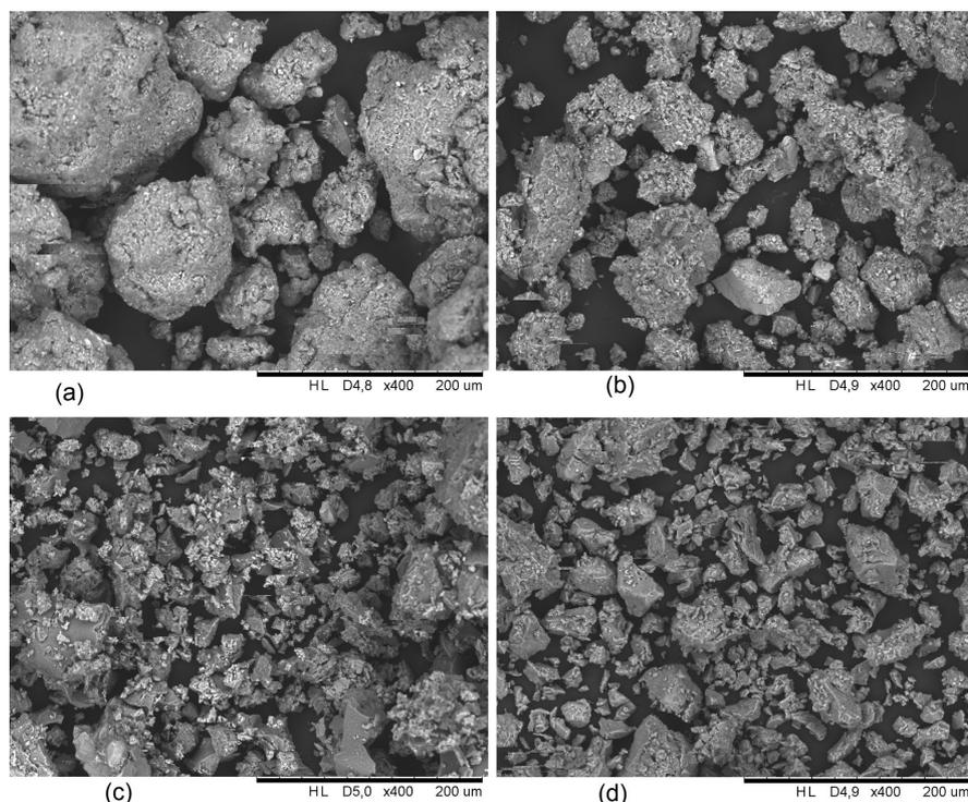
**Figure 6.** SEM photographs of soil before HF treatment in (a) and after HF treatment in (b) and HA before HF treatment in (c) and after HF treatment in (d).
