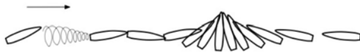
Figure 2. Condensed drawing demonstrating bullet yaw with precession (left), proceeding to tumbling (right). Arrow indicates direction of bullet movement.
