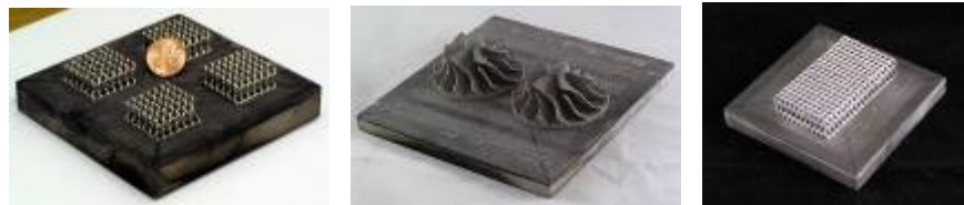
Figure 5. Aluminum Alloys Fabricated Using the EBM Process (Fabricated at North Carolina State University (NCSU))
