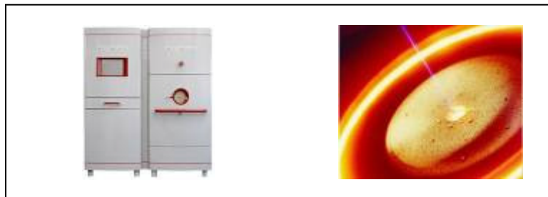
Figure 2. The Arcam S12 EBM Machine and the Electron Beam Material Interaction
