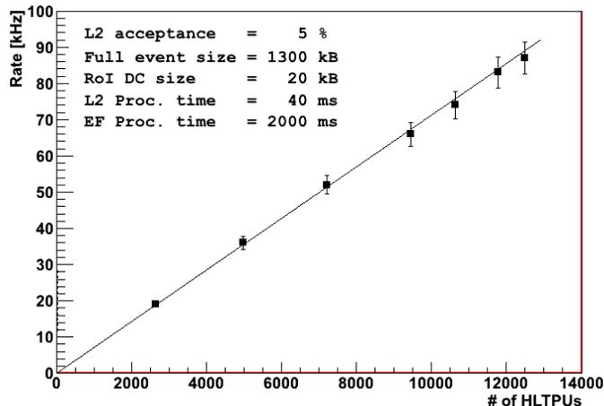
**Figure 4:** Scalability results with new prototype: Total rate vs. number of HLT nodes.
