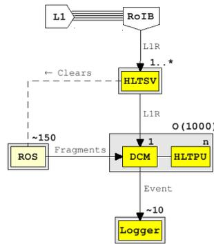
**Figure 3:** New DAQ/HLT architecture
