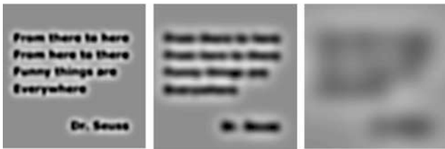
Figure 3 Difference of Gaussians: f_s - f_{3s/2} , s = 8, 16, 44 . 50% gray is zero; dark gray is negative; light gray is positive.
