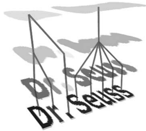
Figure 7 Linked segments in L^- at different scales for part of the Dr. Seuss image.
