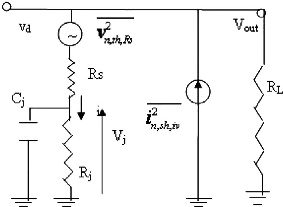
FIG. 3. Diode detector with equivalent noise sources.
