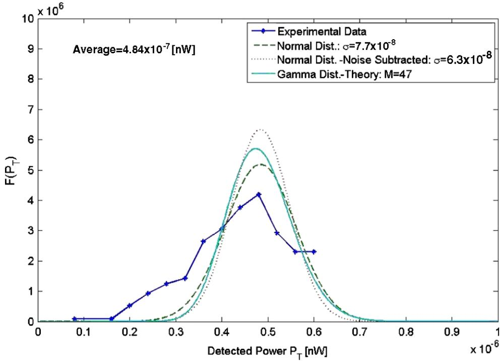
FIG. 5. (Color) Comparison of the experimental data to a Gamma distribution with the theoretical value  $M = 47$ , the Gaussian approximation for the latter, with standard deviation 77 nW and the normal distribution with standard deviation 63 nW
