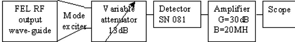
FIG. 2. Measurement setup.
