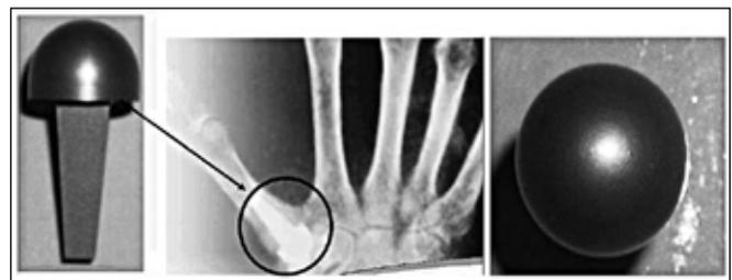
**Fig. 3** - Basal thumb implant produced by EDM from hot pressed  $\text{Si}_3\text{N}_4$ -TiN.
