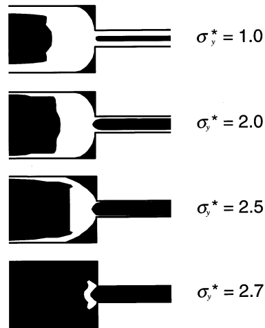
Fig. 21. A sketch of the predicted flow of a Bingham fluid into an abrupt 4:1 orifice for various levels of yield stress, as assessed by \sigma_y^* , from [155]. Dark areas indicate domains where the stress is below the yield stress, i.e. no flow, while white areas indicate domains above the yield stress, i.e. flow.
