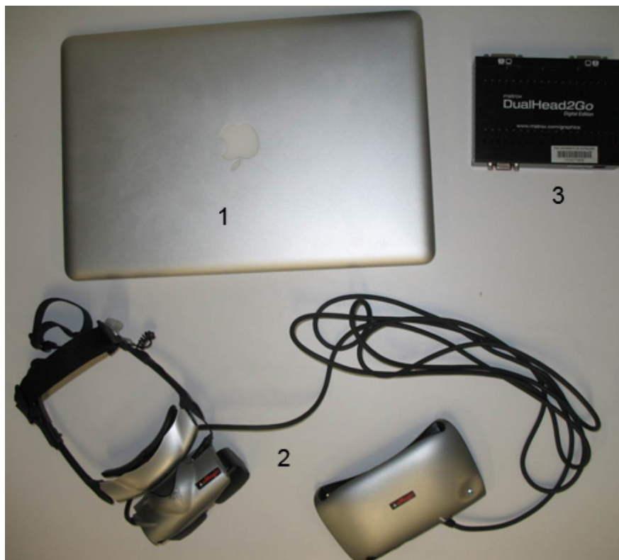
Figure 1. The equipment used for measuring suppression which includes 1) laptop 2) goggles 3) signal splitter.
