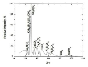
Fig. 1: X-Ray diffraction pattern from the aluminosilicate mineral
