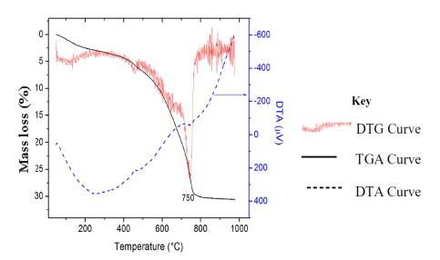
Fig. 3: TGA/DTA curves of the Aluminosilicate clay. TGA Curve DTA Curve
