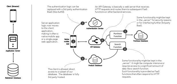
**Figure 9.** Serverless architectures result in a different and less centralized composition of application components and backend services compared with classical tiered application architectures.
