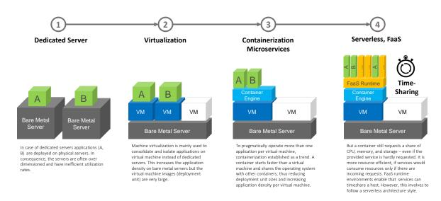
Figure 4. The cloud architectural evolution from a resource utilization point of view.
