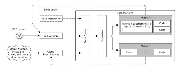
Figure 8. Blueprint of a serverless platform architecture (adapted from [42]).
