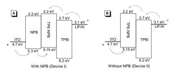
**Fig. 6** Energy level diagrams and device configurations of (A) Device I and (B) Device II. Abbreviation: NPB = N,N'-Di-[(1-naphthyl)-N,N'-diphenyl]-1,1'-biphenyl-4,4'-diamine, TPBi = 2,2',2''-(1,3,5-benzinetriyl)tris(1-phenyl-1-H benzimidazole).
