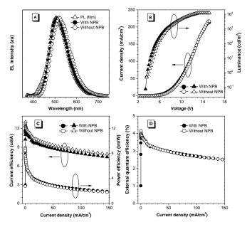
Fig. 5 (A) PL and EL spectra of solid thin film of TPE-NPB. (B) Current efficiency–current density–luminance characteristics of a multilayer EL device of TPE-NPB. Changes in (C) power and current and (D) external quantum efficiencies with the applied current density in a multilayer EL device of TPE-NPB. Device configuration: ITO/(NPB)/TPE-NPB/TPBi/LiF/Al.
