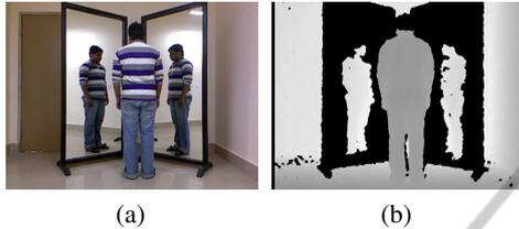
Figure 1: Sample image of a human and his two mirror reflections. (a) RGB View (b) Depth View.
