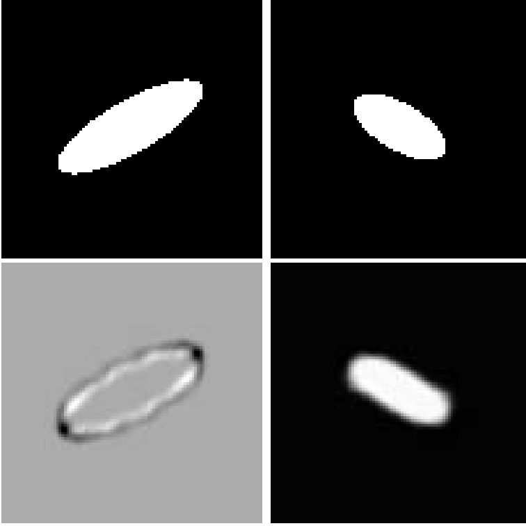
FIG. 1. From top to bottom and from left to right: Initial image, target image, z -coordinate, reconstructed target image.
