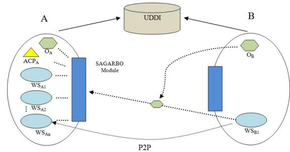
Figure 2: Interoperability Architecture for access control rules generation.
