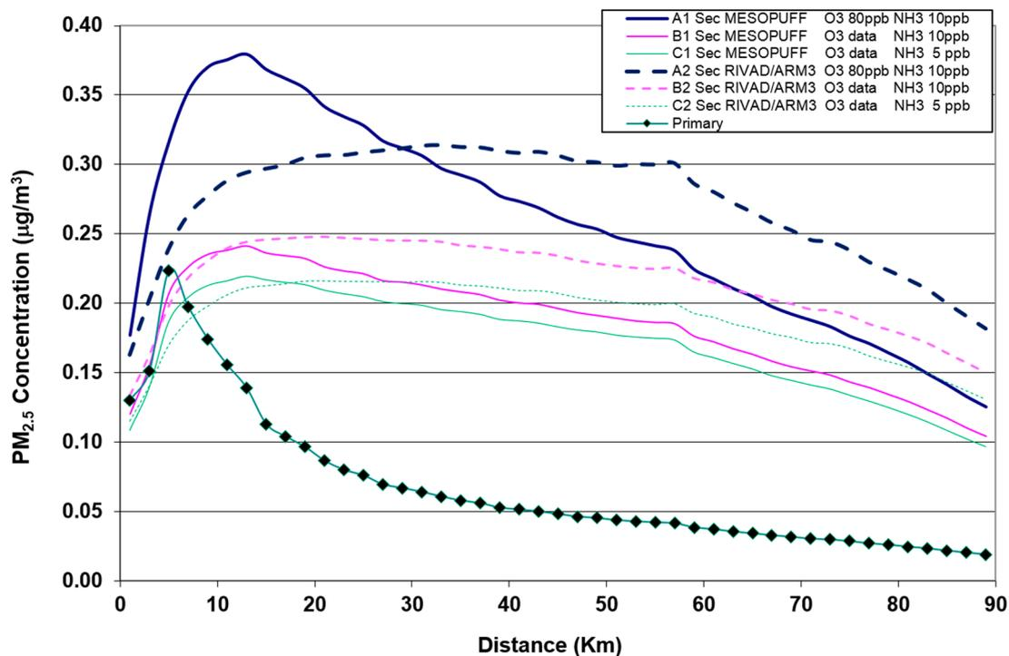
**Figure 4.** Estimated maximum annual average PM<sub>2.5</sub> concentrations ( $\mu\text{g}/\text{m}^3$ ) plotted against distance from the source for different Calpuff runs.
