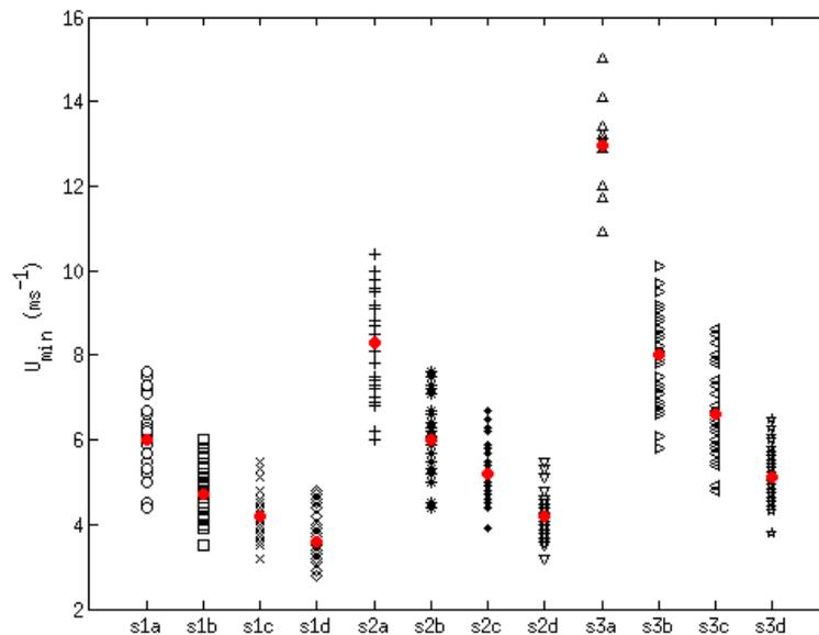
**Figure 5** The minimum annual mean wind speed,  $U_{\min}$ , required for each of the 33 turbines to be economically viable for each of the 12 economic scenarios, as given in Table 1. The red point indicates the median value across all turbine designs.
