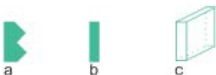
Fig. 1. Symbols used in the drawings and/or gross photographs to indicate the plane of section. a: cutting level parallel to the plane of the picture, b: cutting level perpendicular to the plane of the picture, c: cut level, 3-D.
