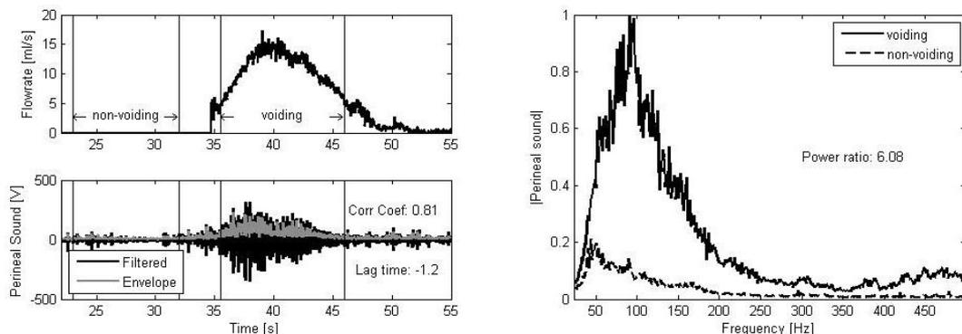
Fig.1. Flowrate (top left) and the filtered sound signal with enveloping curve (bottom left) vs. time. The power spectra (right) during the non-voiding and voiding interval time interval are compared using the power ratio.
