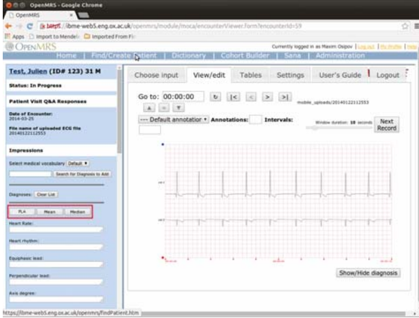
Fig. 4: The OpenMRS Sana encounter UI. The voting algorithm can be triggered by pressing the buttons highlighted in red.
