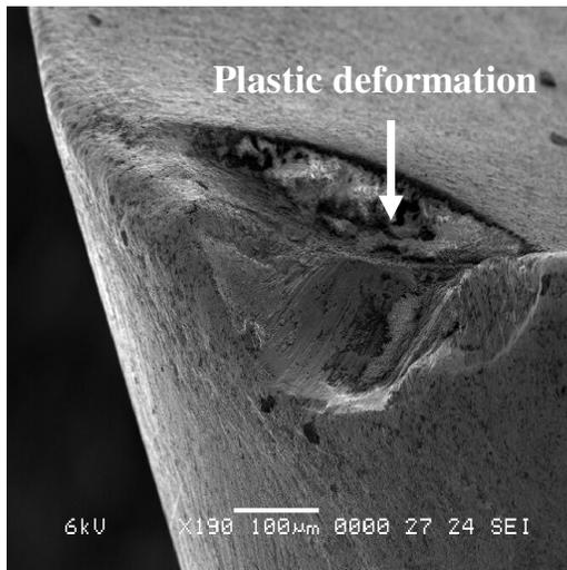
Figure 4.  $V = 160$  m/min, axial DOC = 1 mm, feed = 0.15 mm/tooth
