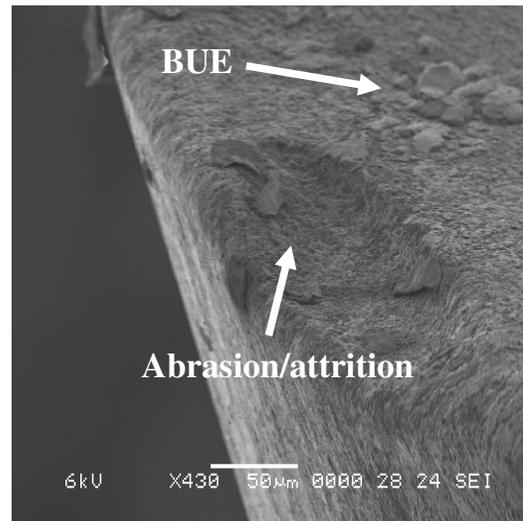
Figure 2.  $V = 70$  m/min, axial DOC = 0.61 mm, feed = 0.088 mm/tooth
