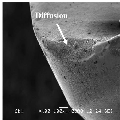
Figure 3.  $V = 127$  m/min, axial DOC = 1 mm, feed = 0.088 mm/tooth
