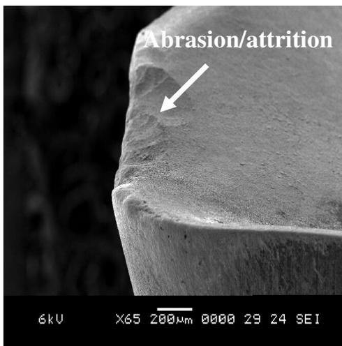
Figure 1.  $V = 39$  m/min, axial DOC = 0.61 mm, feed = 0.06 mm/tooth
