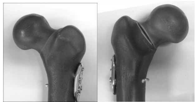
Figure 4. Photograph of femur instrumented with a locking plate (Test B). Left: anterior view; right: posterior view.
