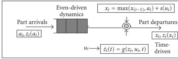
Figure 2.1. A hybrid model for a single-stage hybrid manufacturing system.
