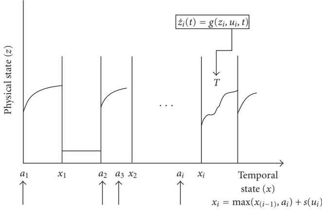
Figure 2.2. The optimal path trajectory of the hybrid system.
