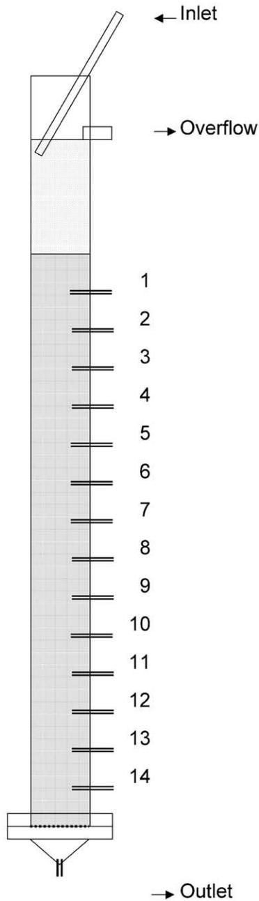
Two columns were prepared. Column I was operated at a pore water velocity of  $1.5 \text{ m day}^{-1}$  and column II at about twice this velocity.
