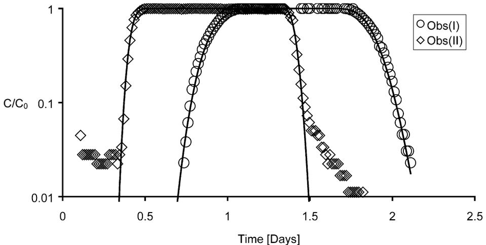
Fig. 2. Measured salt breakthrough curves Obs(I) and Obs(II) from column experiments I and II and fitted breakthrough curves (solid lines).
