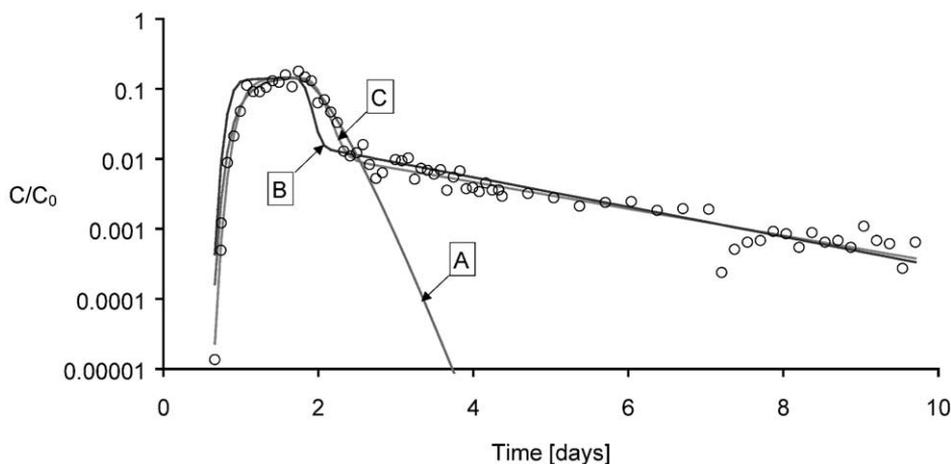
Fig. 3. Measured breakthrough curve (open circles) of MS2 in column I fitted with a one-site kinetic model (curves A and B) and a two-site kinetic model (curve C).
