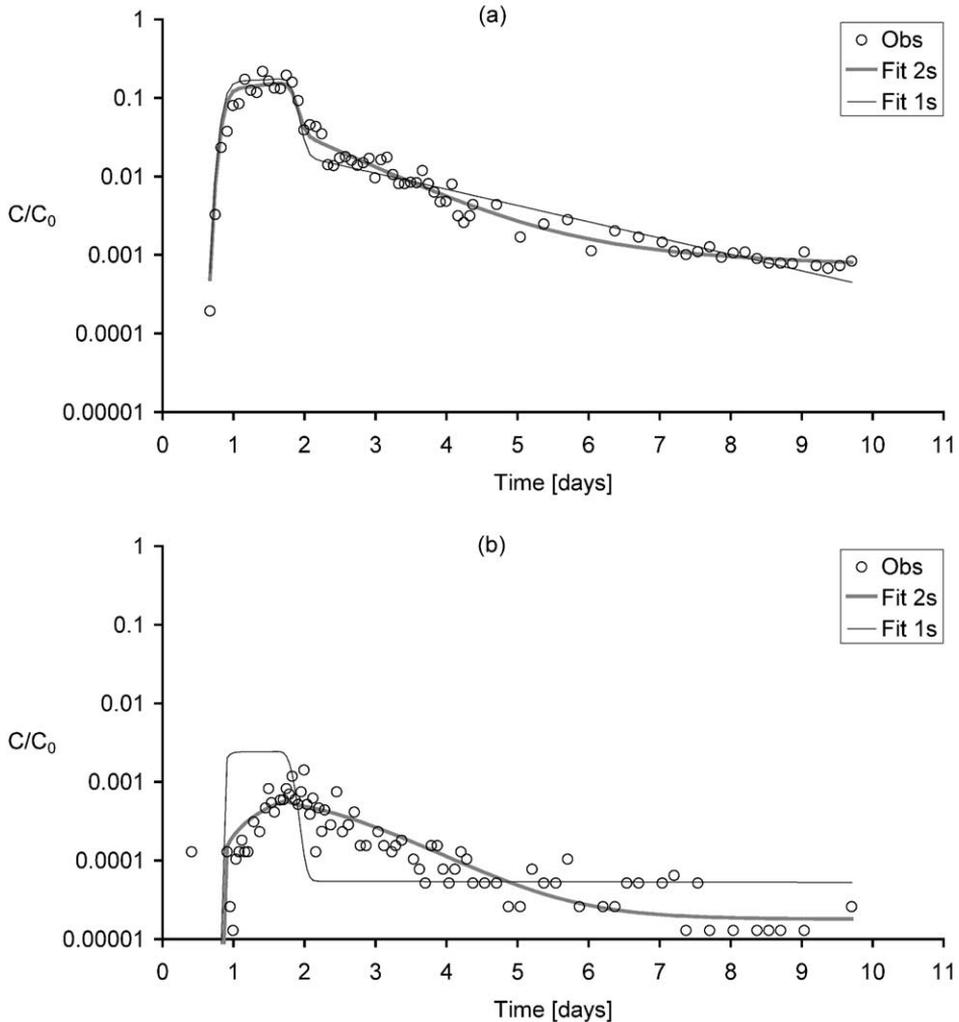
Fig. 5. (a)–(e) Breakthrough curves of bacteriophages. Circles are observations. The solid lines are the one- and two-site kinetic model fit. The dotted lines are the one- and two-site model predictions. In column II two times higher pore water velocity than in column I. (a) PRD1 in column I. (b)  $\phi$ X174 in column I. (c) MS2 in column II. (d) PRD1 in column II. (e)  $\phi$ X174 in column II.
