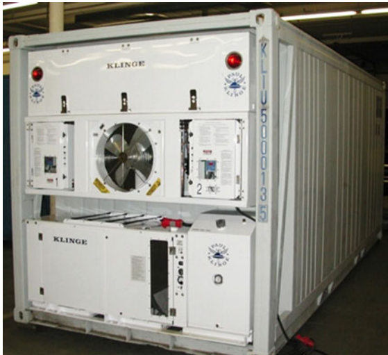
Figure 5.9 Refrigerated container, or reefer, showing refrigeration unit (courtesy of Sarah Klinge, Klinge Corporation).
