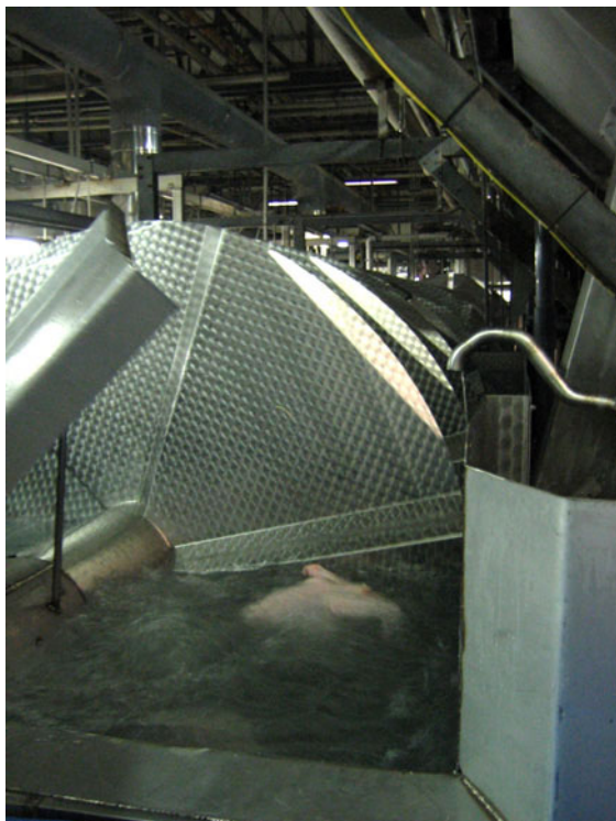
Figure 5.7 Immersion cooling of turkey carcasses.
