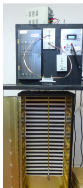
Figure D-2 — Configuration #1 experiments, with emitter EM273. Brass rod is Vertical, accelerometer is in the NADIR direction. Gravity acceleration is oriented towards the accelerometer direction
