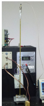
Figure D-4. Configuration #3 experiments with emitter EM273. Brass rod is Vertical, accelerometer is in the ZENITH direction. Gravity acceleration is oriented towards the emitter direction
