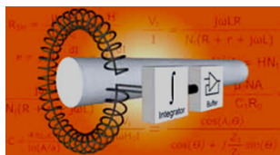
Figure C-2. Principle of a Rogowski coil sensor for measuring a variable current without contact
