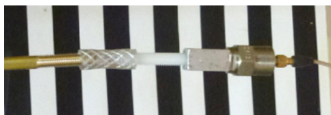
Figure B-1. Miniature accelerometer DJB # 5413 bolted at end of a brass rod with insertion of an insulating separation made of fiberglass. The accelerometer itself is the stainless steel “nut” on the right (12 mm diameter)
