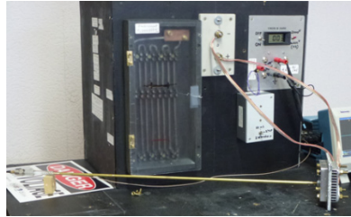
Figure D-3. Configuration #2 experiments, with emitter EM273. Brass rod is Horizontal. Gravity acceleration is PERPENDICULAR to the accelerometer direction
