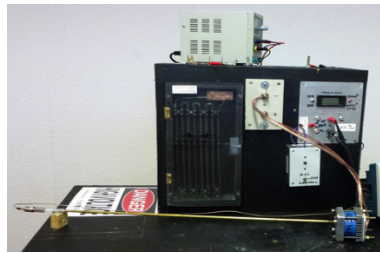
Figure C-5. The 6000 Volts high voltage DC power supply is the grey box, put down on top of the Power box
