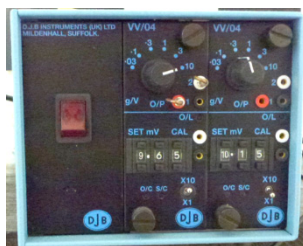
Figure B-2. Double DJB charge amplifier front panel, with calibrated switches
