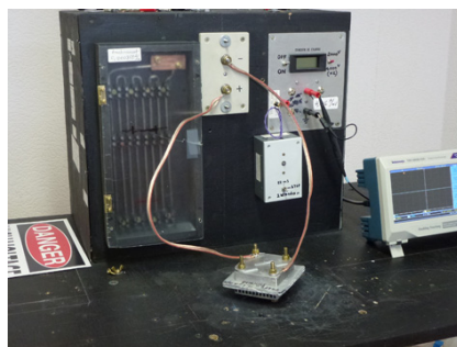
Figure C-4. Emitters are connected to the Power box by two very flexible cables, maintained as distant as possible, to reduce Ampere forces between them. Inverting the connections of these cables allows inversion of the discharge current direction into an emitter. On the right side, onto the Power box, is the digital voltmeter to measure the charge voltage U_0 . The two Rogowski sensor outputs are situated under this voltmeter
