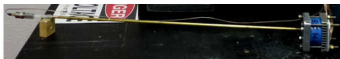
Figure B-4. The accelerometer is bolted at one end of a 623 mm long Brass rod of 6 mm diameter. The other end of the rod is bolted onto the emitter support. The rod introduces a \approx 190 \mu\text{s} delay
