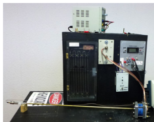
Figure D-1. Configuration #2 experiments, with emitter EM265. Brass rod is horizontal
