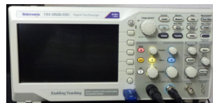
Figure C-6. Experimental results are observed onto a digital oscilloscope Tektronix Model TBS 1052B. It has two channels, Dc to 40 Mhz max frequency, and 1 GHz sample rate. Screen images are recorded on a USB key. Channel #1 is connected to the Rogowski current sensor, with 4.616 Amperes per millivolt calibration factor. Channel #2 is connected to the output of the accelerometer Charge Amplifier with an adjustable calibration. Oscilloscope triggering is generally done by channel #1 (current), when signal is larger than a chosen value
