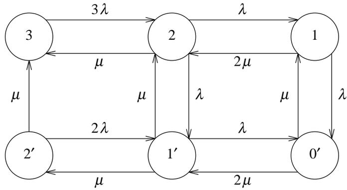
**Figure 6: State Transition Diagram for DLV (Three Replicas on the Same LAN Segment)**
