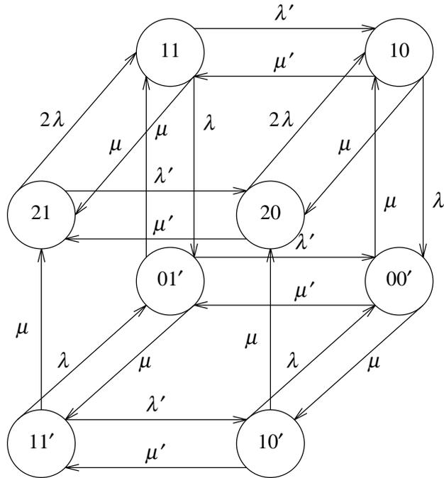
**Figure 7: State Transition Diagram for DLV (Three Replicas on Two LAN Segments Separated by a Gateway)**
