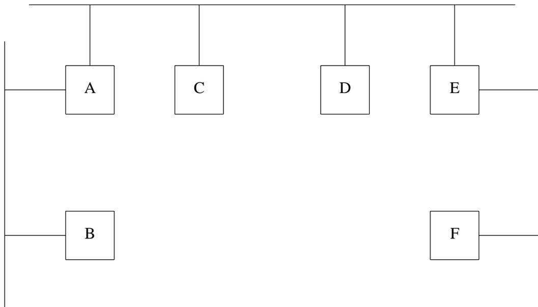
**Figure 1: A LAN with Six Sites on Three Segments**
