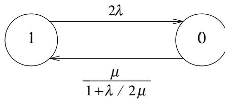
(b) State Transition Diagram for the Equivalent Aggregate Site
