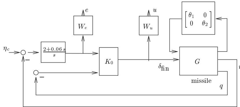
FIG. 1. *Synthesis structure*
