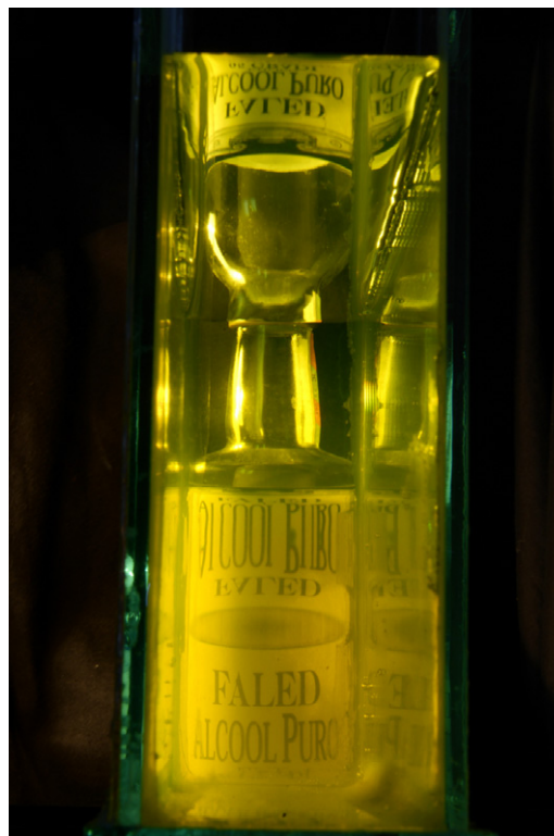
Figure 4. Superior mirage as seen from the point of view of an observer looking through the container.
