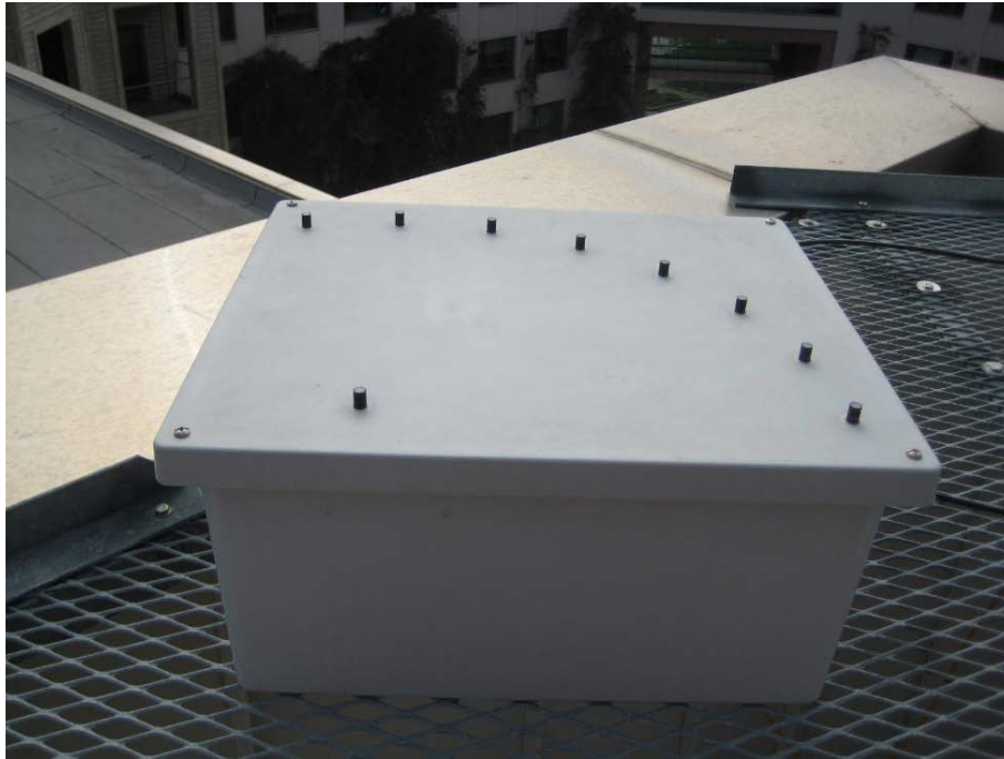
Fig. 2. Cloud speed sensor (CSS). The entire system is contained inside a weather proof enclosure. On the top of the enclosure is the array of nine phototransistors used to measure the variation in solar radiation as clouds pass overhead.
