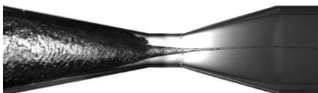
Figure 18 Cavitating vortex filament downstream the SG
