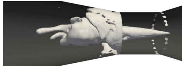
Figure 20 Cavitating vortex captured using the CFD
