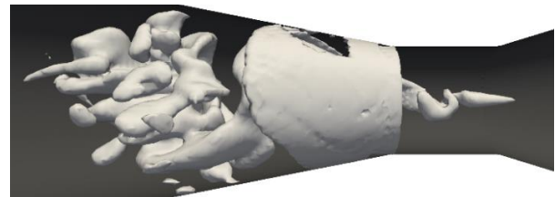
Figure 21 Helical vortex breakdown captured using the CFD
