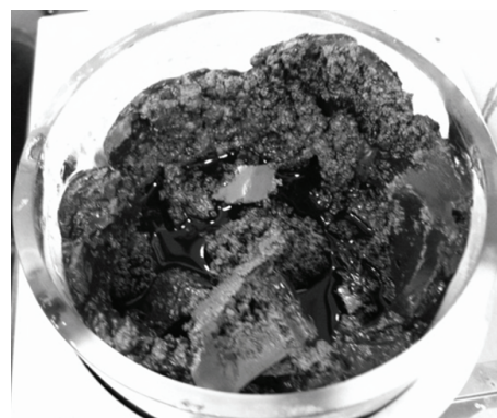
FIGURE 4: Limestone-oil suspension upon addition of 53 mL of water.
